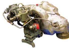
Emergency Power Unit
